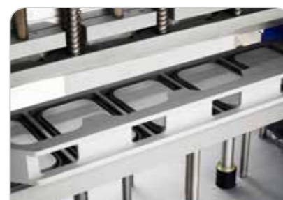
High reliability arm based tray transport
