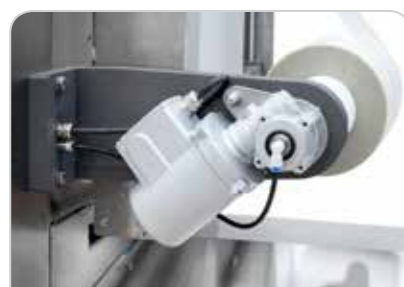
Motorized reel holder with film tension control
